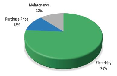
Did you know that a 100 hp air compressor operating 24/7 costs \$63,000 per year in electricity alone! The U.S. Department of Energy (DOE) has determined that electrical costs are 76% of the overall life cycle cost of a compressed air system. Nearly 10% of all electricity consumed in the U.S. powers air compressors. Brabazon's Compressed Air Audits have documented up to 70% in electrical savings and in excess of 80% in maintenance savings for our customers.
